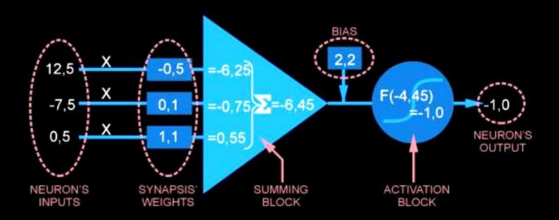
The base units of artificial neural networks are neurons and synapses. Neurons are organized in layers and connected by synapses. Their task is to sum up their inputs and non-linear transfer of the result, which is then transmitted via synapsis with modification by means of the synapsis weights - this signal, in turn, is the input for the next layer of the network
